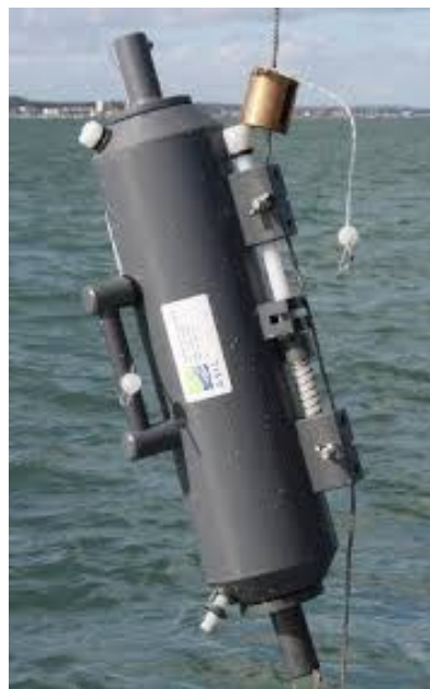
Fig. 4.20 Typical view of a Niskin sampler
